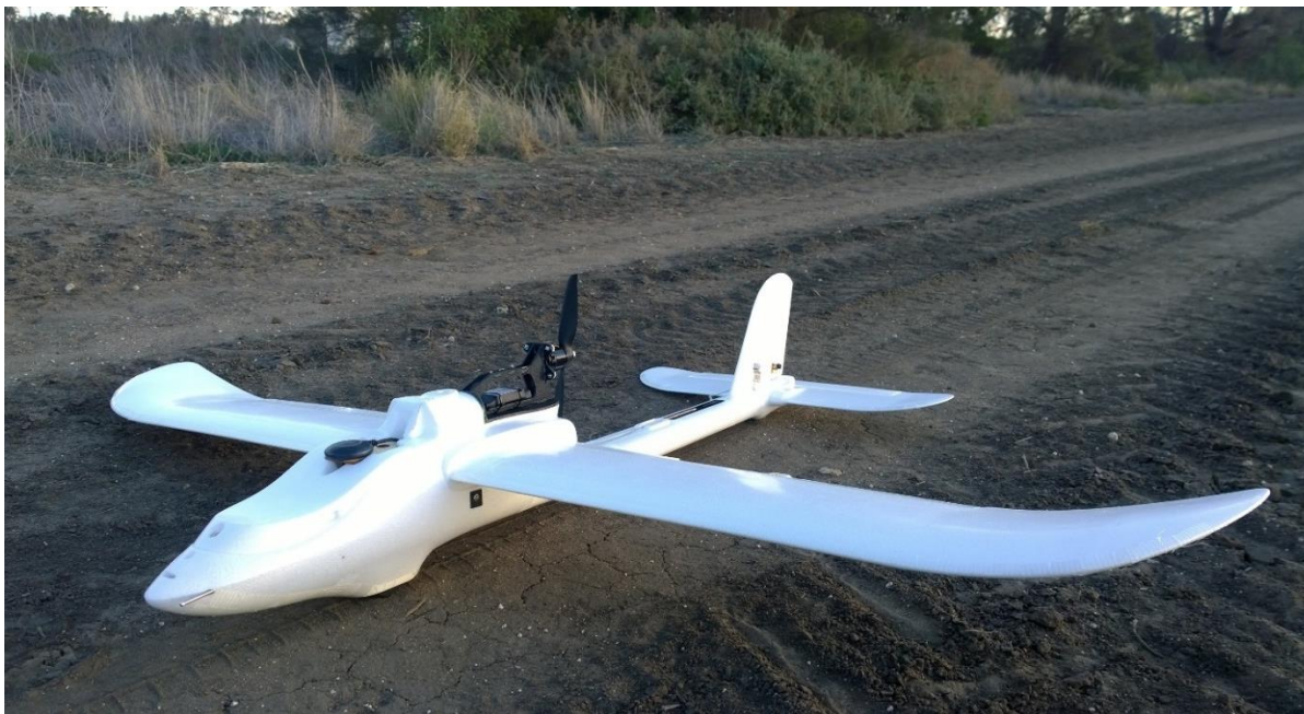
Photo 1: A typical configuration for a fixed wing COTS small UAV, in this case a Finwing Penguin (photo credit: Ben Boughton)
