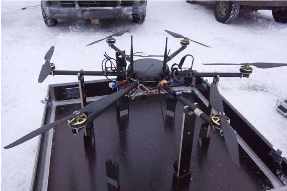
Photo 14: A multi-rotor (hexacopter) COTS small UAV operated by the Ukrainian military's Aerorozvidka unit (photo credit: Aerorozvidka).
