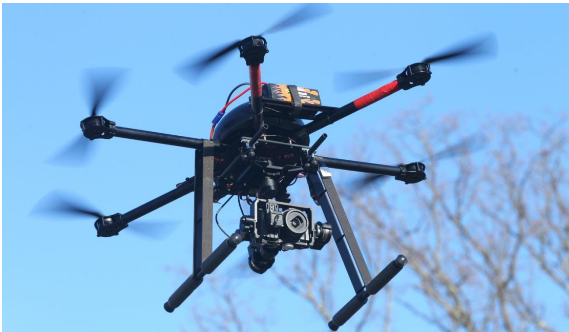
Photo 3: One typical configuration for a multirotor-type rotary wing COTS small UAV, in this case a Gaiu 840H hexacopter (photo credit: Drones Magazine)
