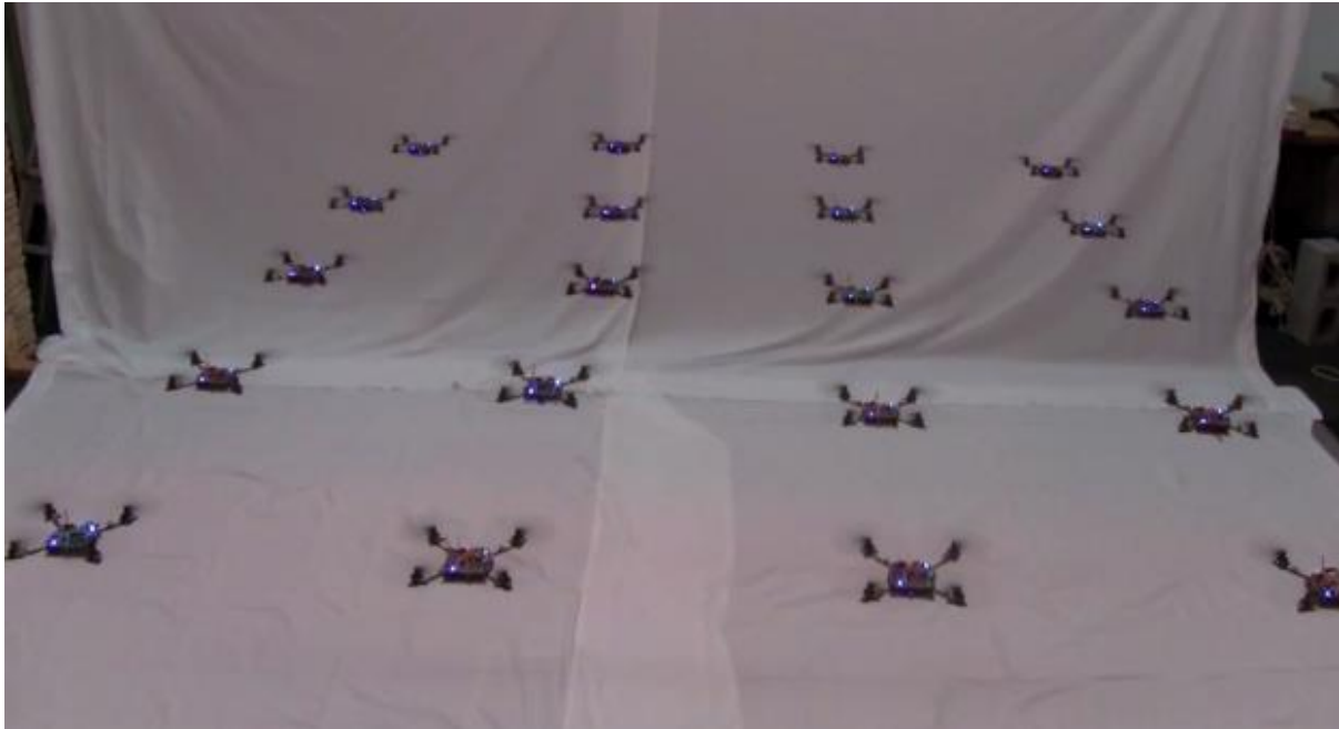
Photo 12: COTS small UAVs demonstrating basic swarming behaviour (photo credit: MIT).
