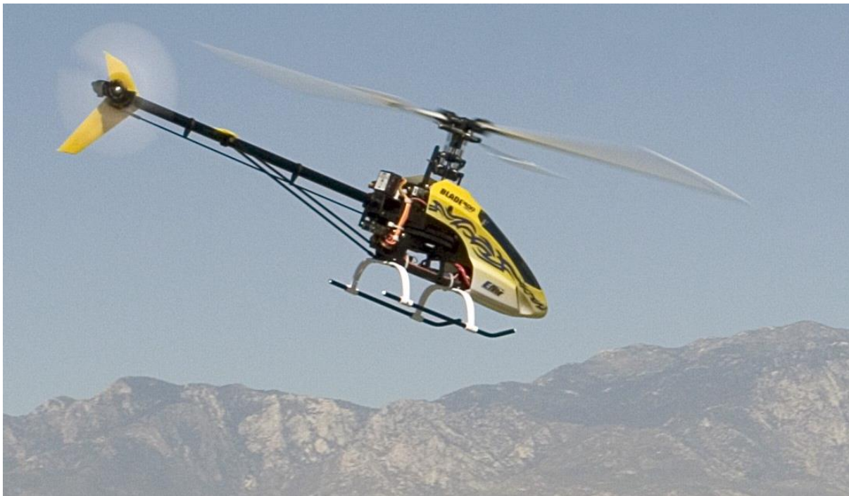
Photo 2: A typical configuration for a helicopter-type rotary wing COTS small UAV, in this case a E-flite Blade 400 3D (photo credit: Wikimedia Commons)
