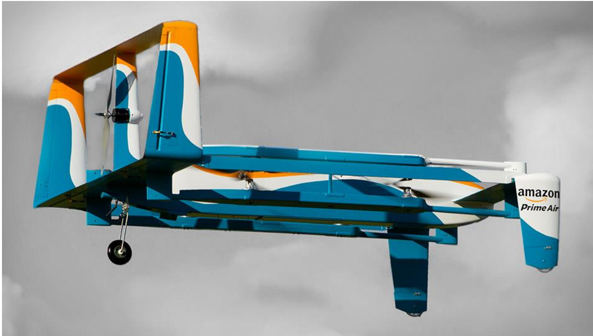
Photo 4: A powered-lift type UAV displayed by Amazon Prime Air (photo credit: Amazon)
