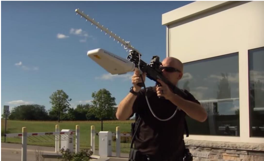
Photo 29: The Battelle DroneDefender counter-UAV system (photo credit: Battelle).
