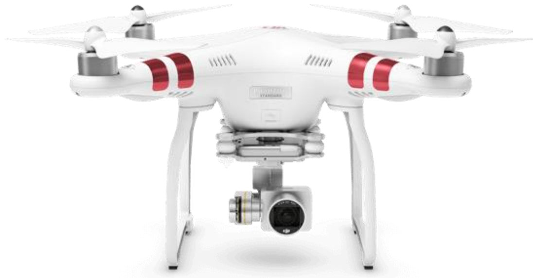
Photo 10: A DJI Phantom 3 Standard rotary wing UAV, which makes extensive use of polymer components (photo credit: DJI).
